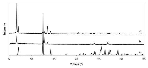
Figure 4: X-ray diffraction patterns. a) Crude theophylline, b) Batch 2, c) SAS 6.
