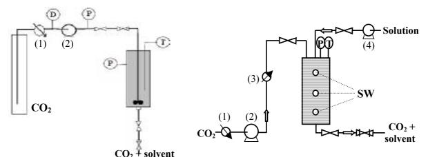
**Figure 1**: Batch set-up. (1) Cooling exchanger, (2) CO<sub>2</sub> pump.
